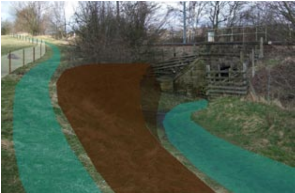
Photograph of the subway under the railway showing how the path would loop around in order to give an easy gradient and how it would be fenced form the field to deal with livestock
