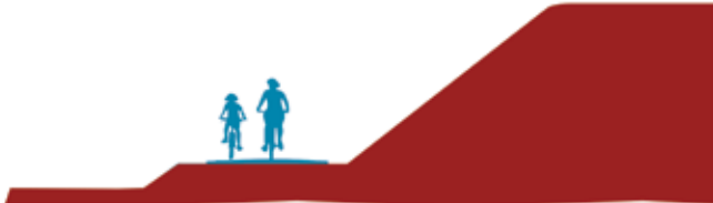
The whole bank then has a wedge 4m wide tapering from full height here to nothing 100m down the line. Here the path position is about 20m from the wall
